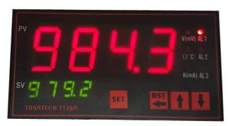
The Trantech TT26D digital process controller is a feature rich display which can accept multiple input types from Analogue mA and voltage signals for pressure and level control systems to RTD and thermocouple inputs for temperature control systems, The TT26D can also be setup for Pulse input to display total pulses or total flow for flow measurement applications. The controller offers a
