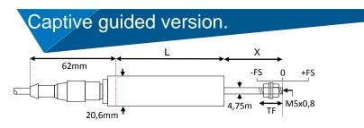
Our captive guided displacement transducer has bearings to guide the armature inside the measurement sensor. Captive LVDTs are for position measurement applications where guidance may be poor and end bearings may be required.
