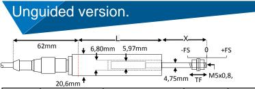
On our unguided LVDTs the armature assembly is a separate component, to make a measurement the user must guide the armature inside the body without touching the sides. Unguided position measurement transducers are appropriate where external guidance is available and give truly non-contact operation
