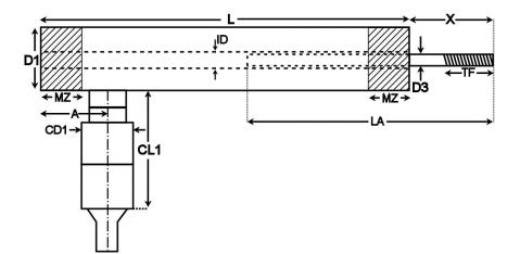
A = 48mm CD1 = 35mm CL1 = 92mm D1 = 38,1mm D3 = 10mm ID = 13mm
